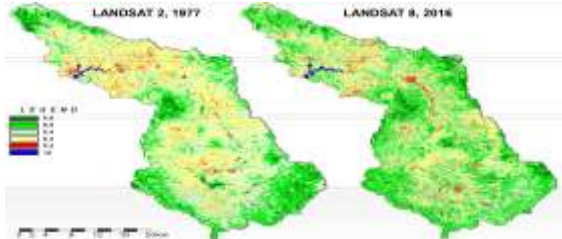
Fig. 2: Potential erosion rate in the catchment between June 1977 and June 2016, calculated from Landsat 2 and Landsat 8 imagery with SAGA GIS v4.1.
