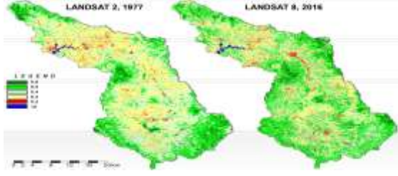
Fig. 2: Land cover change in the catchment between June 1977 and June 2016, calculated from Landsat 2 and Landsat 8 imagery with SAGA GIS v4.1.
